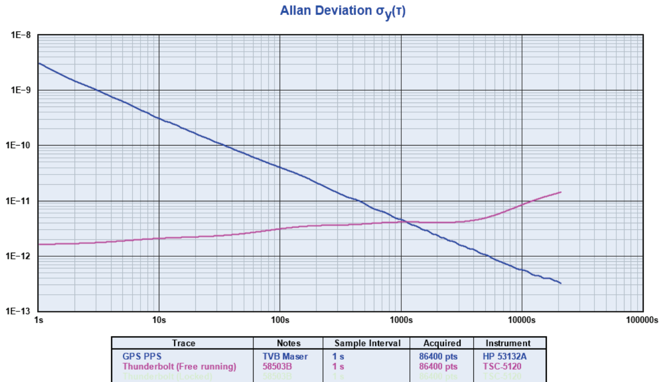
Figure 38: Allan Deviation Intercept of GPS and OCXO 25
