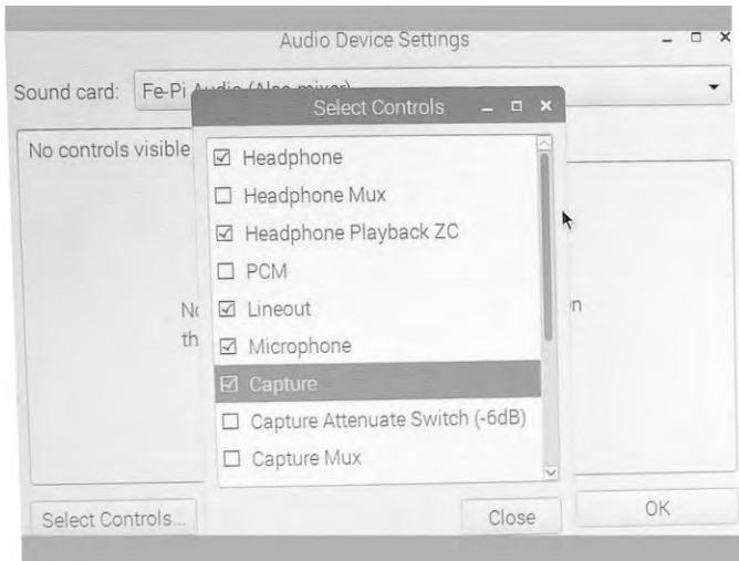
Settings. Set the Fe-Pi Device that is listed besides the bcm2835 ALSA as the default device. To gain access the volume controls press the “Select Controls” button and then select the controls as shown in the picture left. Set all the “Capture“ devices to max for the RF-Seismograph setup.
