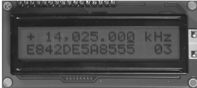
**Figure 13 — The first line of the LCD shows RFREQ.**
