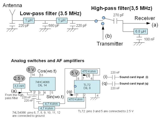
The system below supplies two signal in quadrature at a frequency f0 equal to the quarter of the frequency of the crystal oscillator (i.e. here: 14.31818/4=3.579545 MHz). These signal are not, strictly, sinusoidal (Cos(wot)/Sin(wot)) but rather TTL signals, so with harmonics which are not annoying because removed downstream (either by the TL72 amplifier and the anti-folding filter of the sound card in RX or by the low-pass filter in TX).
