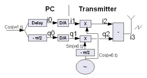
The « Delay » is done with an « all-pass filter ». It simply compensates the delay (φ) introduced by the « π/2 » phase shifter. This one introduces a necessary delay, because the goal is not to shift a pure carrier but to shift an AF band. Consequently, it is necessary to use a phase shifter filter, introducing some inevitable delay.
