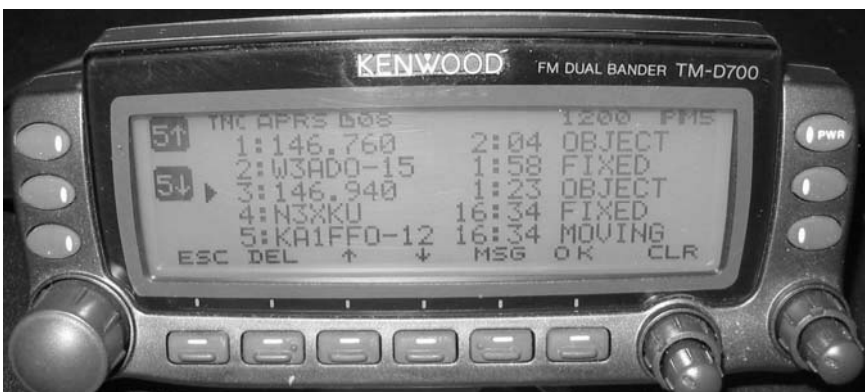
Figure 5. By using the recommended local voice repeater frequency as an APRS object name, these recommendations show up for the mobile traveler whenever he enters a new area. This D700 shows the most recently received 146.76 is in direct range. The older 146.94 has moved down the list since it was heard 35 minutes earlier.
