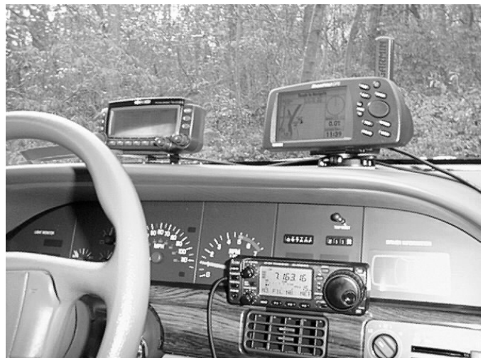
Figure 1. W4HFZ's typical mobile setup includes VHF, UHF, HF, a GPS and APRS.
