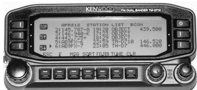
Figure 4. The new D710 mobile radio adds a column for frequency info and also has a TUNE button for instant QSY to contact one of those stations. The first three objects are nearby voice repeaters, and AB9FX has two stations nearby, Another D710 monitoring 52 and his D7 HT monitoring 446.000.
