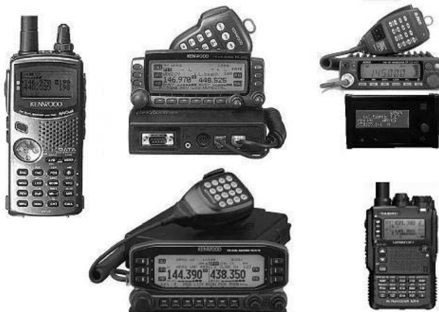
Figure 2. For over 10 years, there have been a variety of fully integrated APRS radios as shown here. Shown left to right, first was the D7 and then D700. Then the DR-135 with add-on HamHUD to give it an APRS display capability, and then in 2007 the fully capable D710 and recently the VX8R.
