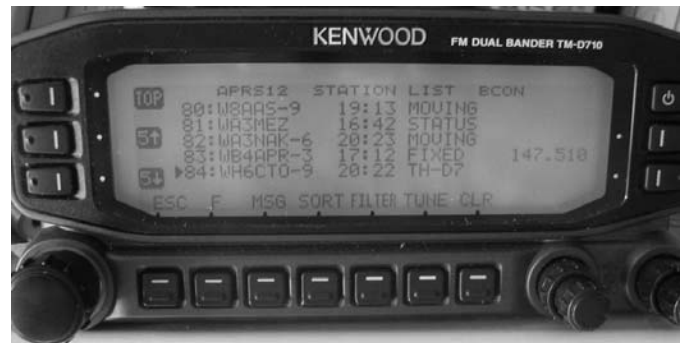
Figure 3. This D710 display list was sorted by callsign (W’s) and station WB4APR-3 is a fixed station reporting that he is monitoring 147.51 MHz. Clicking on this list will reveal 3 more pages of info on that station, or you can just press TUNE button and talk to him if his repeater or frequency is in range.
