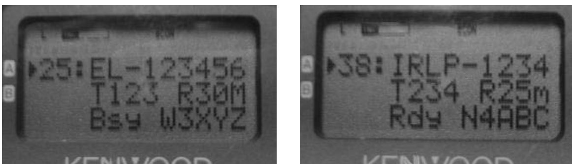
Figure 6. Nearby Echolink and IRLP nodes can also beacon their Position, Frequency, Tone and their node numbers. This makes mobile-to-mobile dial-up global communications possible. These displays show the node number and tone., but the second line should actually be the frequency.
