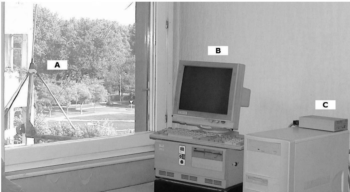
Figure 8. Main parts of the JNOS mailbox subsystem in the home LAN.
