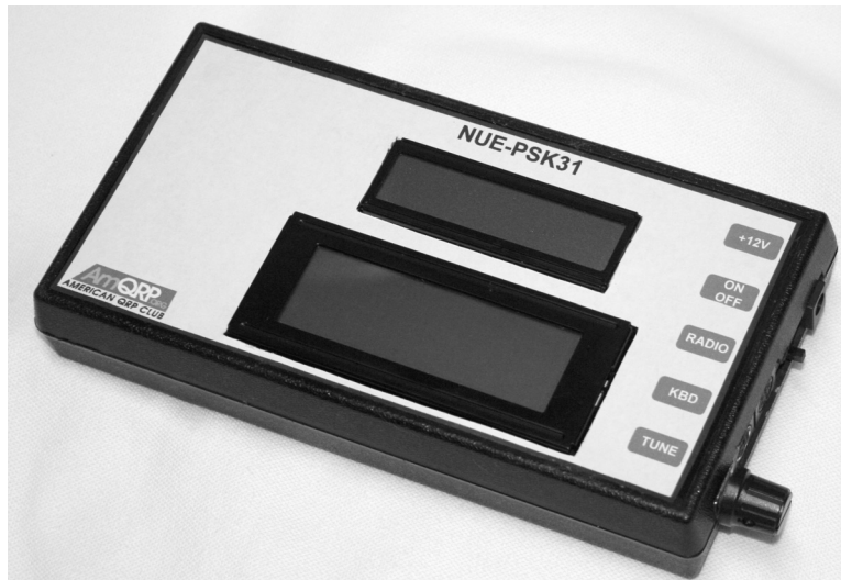
Photo 1: NUE-PSK31 in mating plastic enclosure. Powered by 9V battery contained within (~100ma current draw), with connectors and controls on right side panel.
