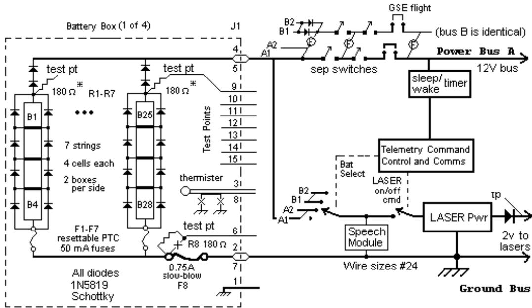
Figure 3. ANDE Battery System Schematic showing the one of the four parallel battery packs and the battery switching arrangement for the laser power system.
