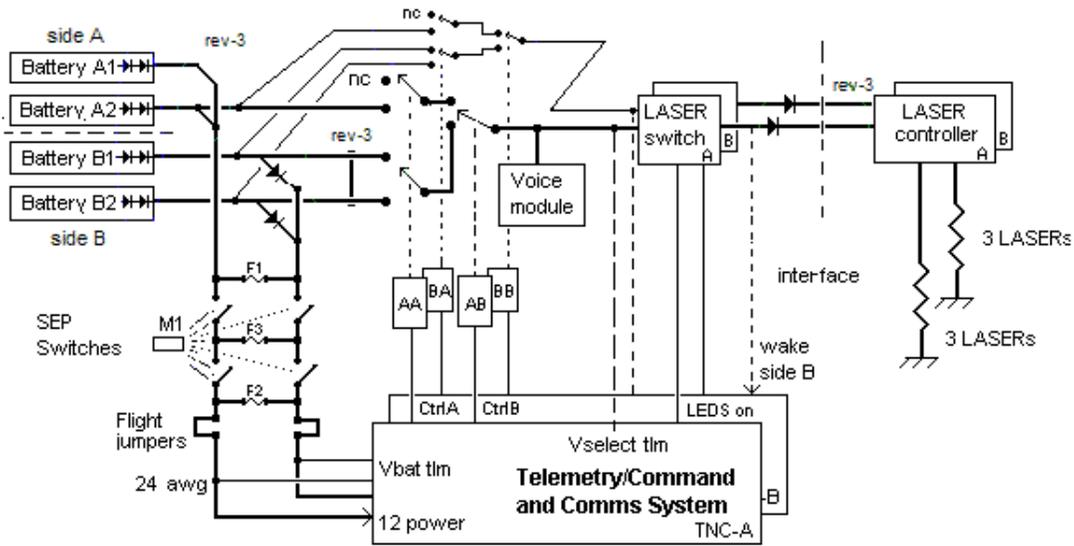
The TCC system is always redundantly powered by all battery strings. But the LASER load was to be separately powered from one battery pack at a time via RYA or RYB. But to get enough current, the A and B systems had to be paralleled. The C1-C3 lines are the 3 command switches per TNC controller. A is primary, B is backup. All power system wiring is #24 awg.
