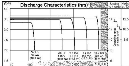
Figure 5. Lithium Primary Cells discharge curve.
