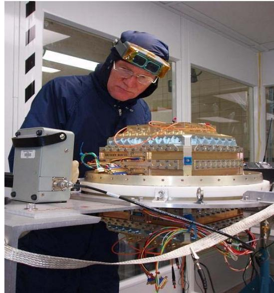
Figure 6. The photo above shows the identical top and bottom stacks. Each stack consists of two battery trays and then a Comm tray and topped by a smaller laser module.
