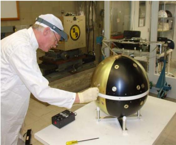
Figure 1. The ANDE spacecraft during final tests at the Naval Research Labs in Washington DC. This photo shows the final tweaks of the antenna matching network to match the sphere to the 145.825 MHz operating frequency.
