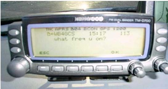
Figure 8. The front panel APRS message capability of the Kenwood D700 radio. Messages can be up to 64 characters in length.
