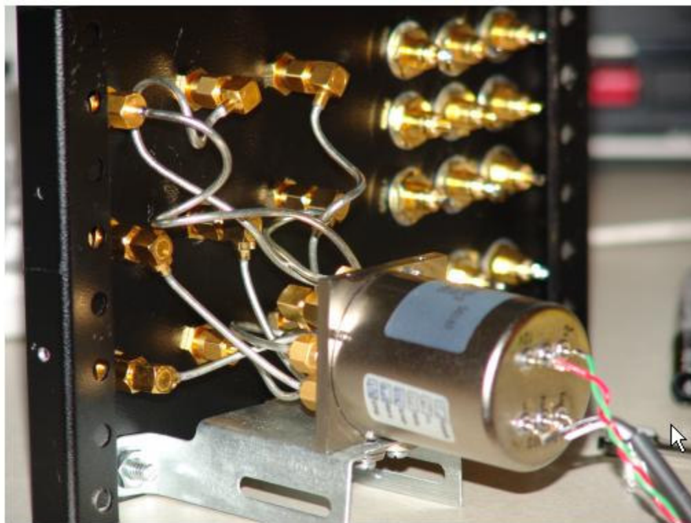
Closeup of SMA Jumpers to Rear Panel Bulkheads
